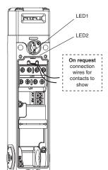
• This switch may be supplied with two green LEDs to show from the outside of the switch the solenoid supply state. Wiring is not necessary. On request, it is also available a version with the two LEDs in different colours showing the contact state.
