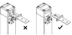
Attention: Periodically check the correct alignment between the switch and the respective actuator. The actuator must not knock on the outside of the actuator inlet area, and must not be used as a centring device for the mobile
