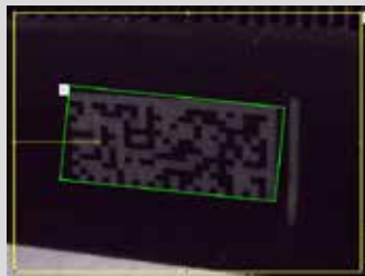
Code with low contrast This is made readable by the high tolerance to weakly contrasting codes.
