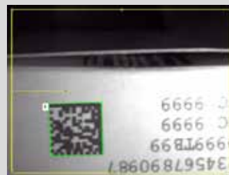
Printed codes on pharmaceutical packaging It is possible to search for both ECC200 or bar codes (e.g. EAN 13) simultaneously. In addition to code reading, the presence of optical characters can be inspected using object detection.
