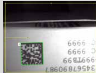
Printed codes on pharmaceutical packaging ECC200 or bar codes (e.g. EAN 13) can be searched for simultaneously. In addition to code reading, the presence of optical characters can also be checked using object detection.
