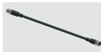
Extension cable with M12 connectors Polyurethane connector body Protection degree IP67 Gold-plated contacts (resistance < 5 mΩ) Self locking ring nut
