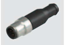
M12 terminating plugs for series connections Polyurethane connector body Protection degree IP67 Gold-plated contacts (resistance < 5 mΩ) Self locking ring nut
